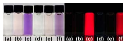
Figure 3. Photographs showing the color changes (left) and emission enhancement (right) in the absence of Hg(II) ion for cis -2 (a) and trans -2 (d), and in the presence of 1.5 equiv of Hg(II) ion for cis -2 (b) and trans -2 (e) and in the presence of excess amount of Hg(II) ion for cis -2 (c) and trans -2 (f) in MeOH.
